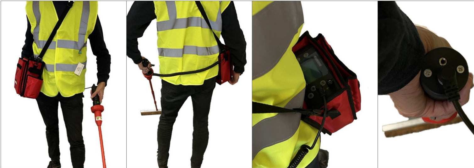
The interconnect cable is worn behind the body
